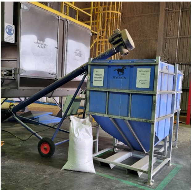
Blue Stakka bins are replacing single-use bulka bags for the transport of raw materials on-site.
